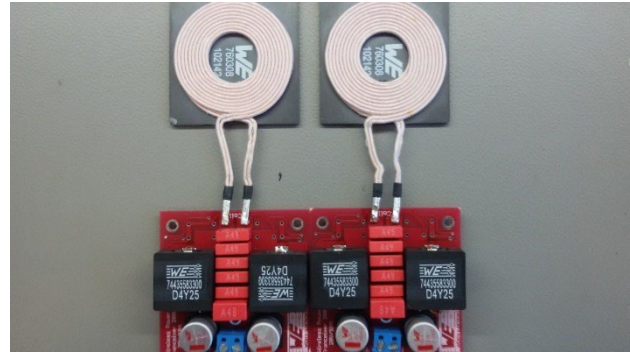
Figure 7: Measured circuit ( V_{in} = 20\text{ V}_{DC} ; P_{out} = 100\text{ W} ) for a 6.5 mm air gap.
